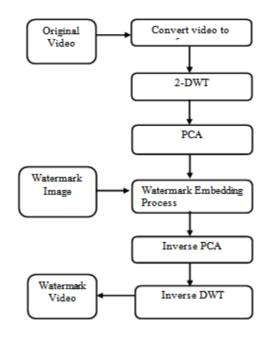
Figure c Flowchart of watermark embedding process
